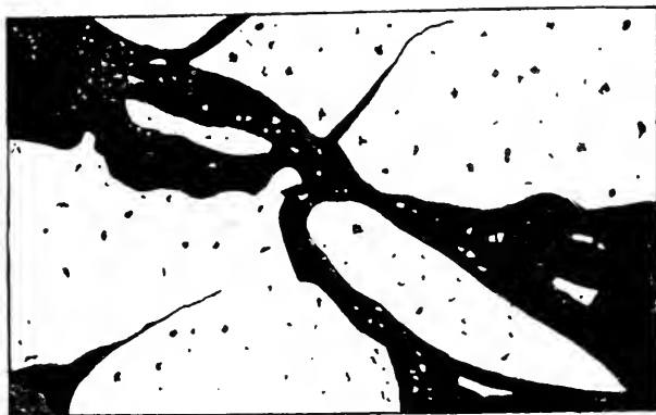
Fig. 25—Shows relation of sulphides to norite hanging wall. White represents norite; black represents sulphides. Eighth level, Creighton mine, Sudbury area, Ontario. Width of face 15 inches. The drawing illustrates the fact that the sulphides were introduced after the norite had solidified.
